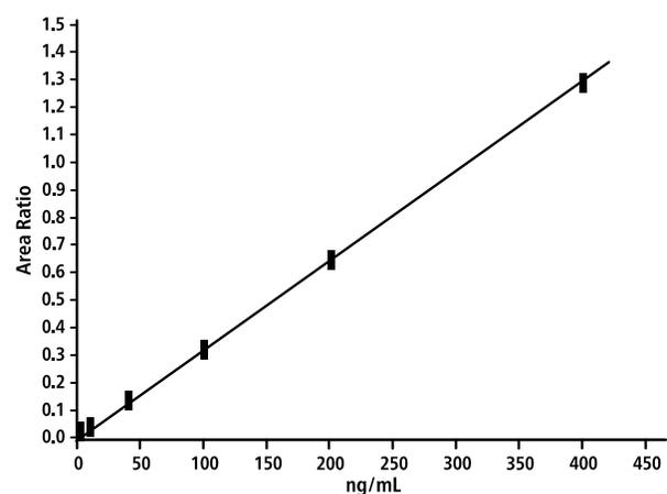
Figure 2: Simazine calibration curve
